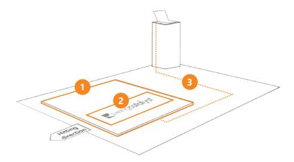
For a more permanent installation, we recommend building the Balance Plate into a mat of artificial turf.
