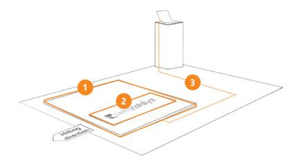
For a more permanent installation, we recommend to build the Balance Plate into a mat of artificial turf.
