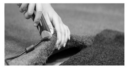
Cut an incision under the mat to make room for the USB cable. The USB cable should come out on the heel side for right handed golfers, and placed under the mat. Connect the USB to the computer.
