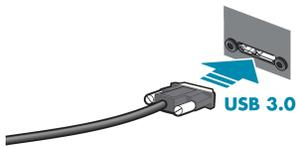
Plug the interface cable into the host controller card and the camera. The cable jack screws can be used for a secure connection.
