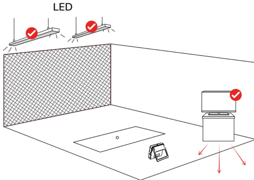
Noisy electronic devices in front of the unit may cause poor tracking performance.
