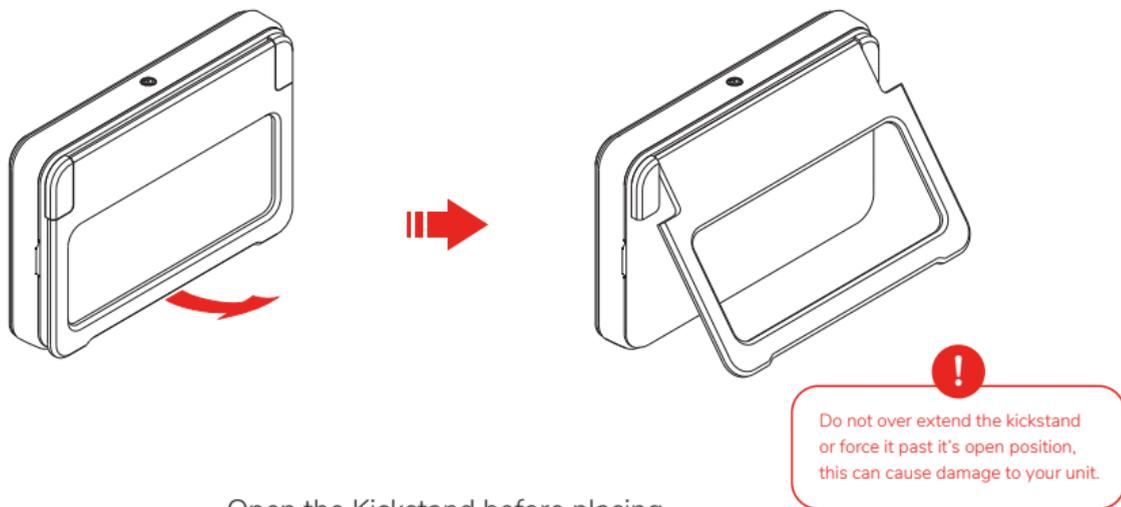
Open the Kickstand before placing.
