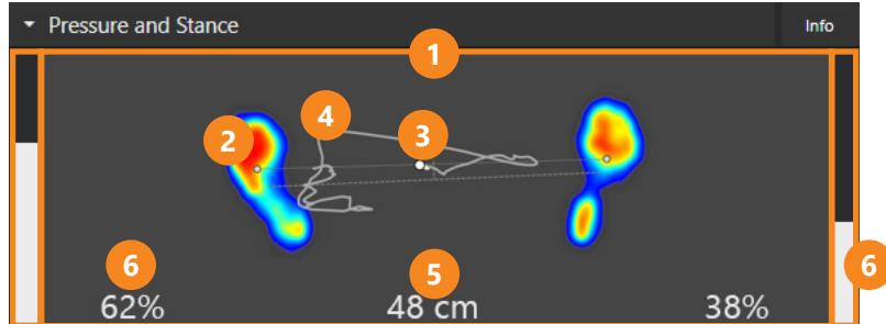
The top layer of the Swing Catalyst 3D Motion Plate consists of more than 2000 high-resolution sensors and measures the pressure applied to the ground by the golfer. The Balance Plate provides information on center of pressure, stance width, and pressure distribution between the feet. This information can be seen in the *Pressure and Stance* data box in the Swing Catalyst software:
