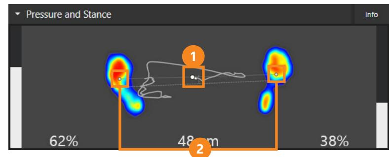
The white circle indicates the position of the total CoP, which is affected by the pressure distribution. For example, movement of the CoP toward the lead foot indicates a relative increase in pressure under the lead foot.
