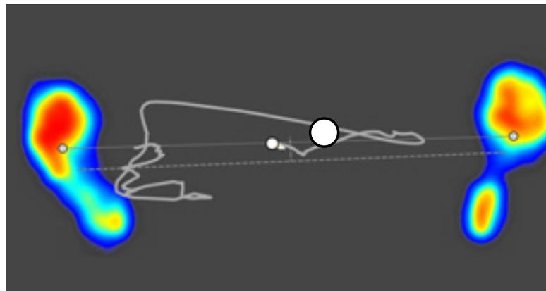
The colored footprints in the box indicate the contact that is present between the shoes and the plate. Different amounts of pressure are shown by different colors, with "colder" colors such as blue representing areas of low pressure and "hotter" colors such as red representing areas of high pressure.
