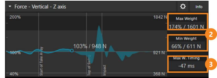
2 The Max Weight and Min Weight values on the right side of the box show the magnitude of maximum and minimum vertical force achieved during the swing, relative to body weight.
