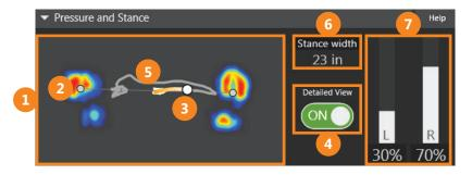
The Swing Catalyst Balance Plate consists of more than 2000 high-resolution sensors and measures the pressure applied to the ground by the golfer. The Balance Plate provides information on center of pressure, stance width, and pressure distribution between the feet. This information can be seen in the *Pressure and Stance* data box in the Swing Catalyst software:
