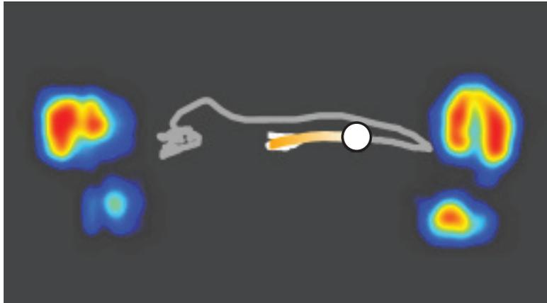
The colored footprints on the left side of the box indicate the contact that is present between the shoes and the plate. Different amounts of pressure are shown by different colors, with blue representing the least pressure and red the most.
