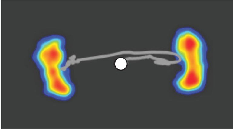
A flat-soled shoe, on the other hand, will typically show a more even distribution of pressure over the foot. This is because the force exerted on the ground by the golfer is spread over a larger area. In this case, specific points of high pressure will be more dependent on where under the foot the golfer exerts the most force on the ground.
