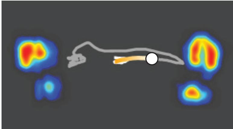
Pressure coloring will reveal tendencies to lean on specific parts of the foot during the swing. This is most obvious when there are differences between the heel and forefoot or between the inside and outside of the foot. Tendencies to lift parts of the foot off the ground are revealed by a lack of pressure coloring.
