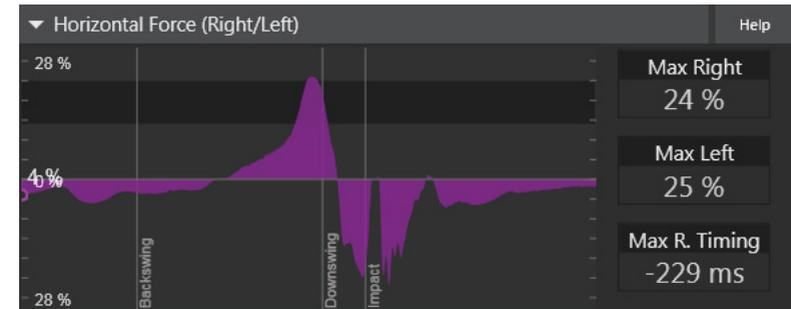
The shape of the horizontal force (right/left) graph shows how the golfer's dominant direction of force changes throughout the swing. An increase in the direction of the right foot indicates either movement to the left or resisting movement to the right, while an increase in the direction of the left foot indicates either movement to the right or resisting movement to the left.
