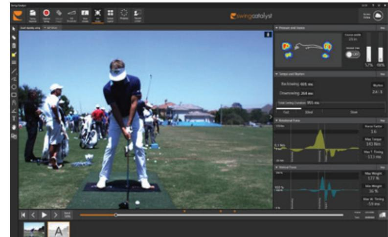
The bottom layer of the Swing Catalyst 3D Motion Plate is a 6 component force plate, measuring forces in three dimension and torques about three corresponding axes. The force plate component provides both graphical and numerical information on torque, vertical force, and horizontal force produced at the feet. This information can be seen in the various force data boxes in the Swing Catalyst software. All force data is fully synchronized with the video images.
