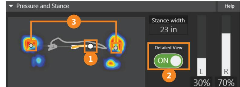
The white circle indicates the position of the CoP, which is affected by the pressure distribution. For example, movement of the CoP toward the lead foot indicates a relative increase in pressure at the lead foot.
