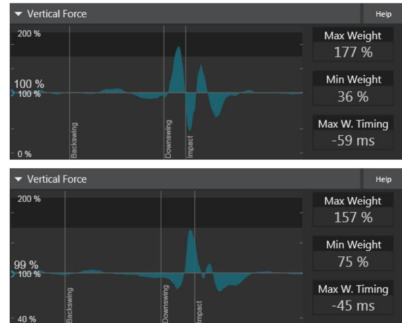
The shape of the vertical force graph shows how the golfer's vertical acceleration of body mass (experienced weight) changes throughout the swing. An increase in the graph indicates either upward movement or braking of downward movement, while a decrease in the graph indicates either downward movement or braking of upward movement.
