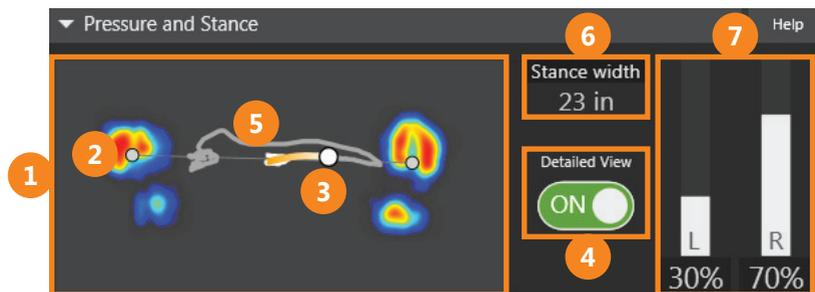
The top layer of the Swing Catalyst 3D Motion Plate consists of more than 2000 high-resolution sensors that measure the pressure applied to the ground by the golfer. This pressure plate provides information on center of pressure, stance width, and pressure distribution between the feet. This information can be seen in the Pressure and Stance data box in the Swing Catalyst software:
