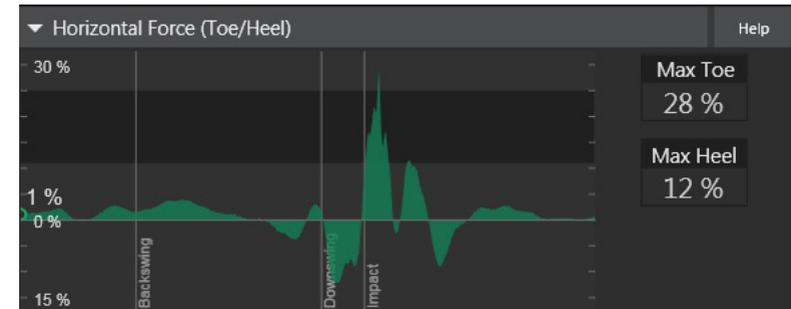
The shape of the horizontal force (toe/heel) graph shows how the golfer's dominant direction of force changes throughout the swing. An increase in the direction of the toe indicates either backward movement or resisting forward movement, while an increase in the direction of the heel indicates either forward movement or resisting backward movement.
