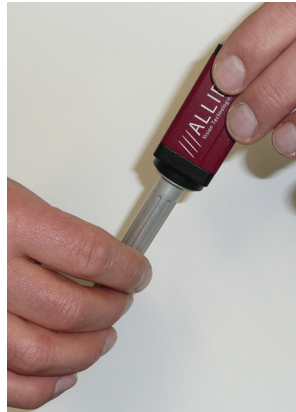
Figure 3: Removing IR cut filter/protection glass using special tool (E9020001)
