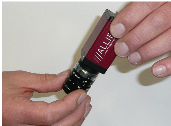
Figure 1: Hold camera like this while changing the lens/removing the dust cap of a camera
