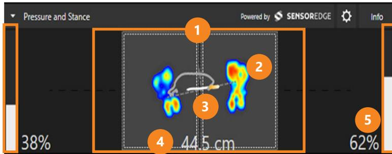
The Swing Catalyst Balance Plate consists of more than 2000 high-resolution sensors and measures the pressure applied to the ground by the golfer. The Balance Plate provides information on center of pressure, stance width, and pressure distribution between the feet. This information can be seen in the *Pressure and Stance* data box in the Swing Catalyst software:
