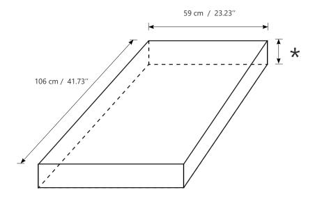
★ The height depends on the height of the turf you have selected. The total height of turf and floor construction should be approximately 9.2 cm / 3.62 inches. Please measure the total height of the 3D Motion Plate and logo mat beforehand.
