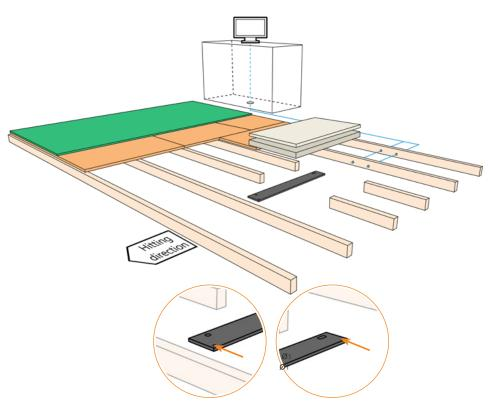
ø1: Mounting holes. Use screws to fix mounting rail to the floor.
